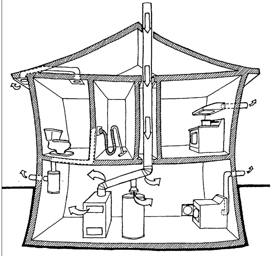
to be reversed. In houses where the “on” cycle is short and the chimney is not insulated, this type of start up spillage may occur frequently, since the chimney has little opportunity to heat up and establish a good draft. Because the combustion products during start-up are particularly dirty, even minor spillage of this type should be considered undesirable.
