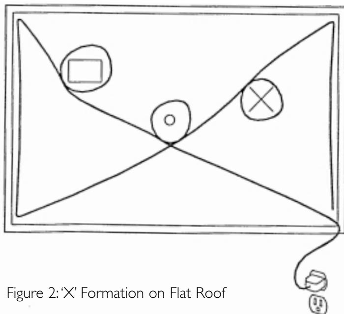
Figure 2: 'X' Formation on Flat Roof
